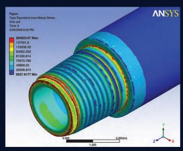
The FEA analysis confirms the reduced peak stresses and SCF (stress concentration factor) in the thread roots. The benefit is a more robust connection and superior fatigue resistance.
