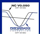
Larger Performance Technology Plus Connections have even greater reduced Tool Joint Stiffness – from 20% to 39%.
